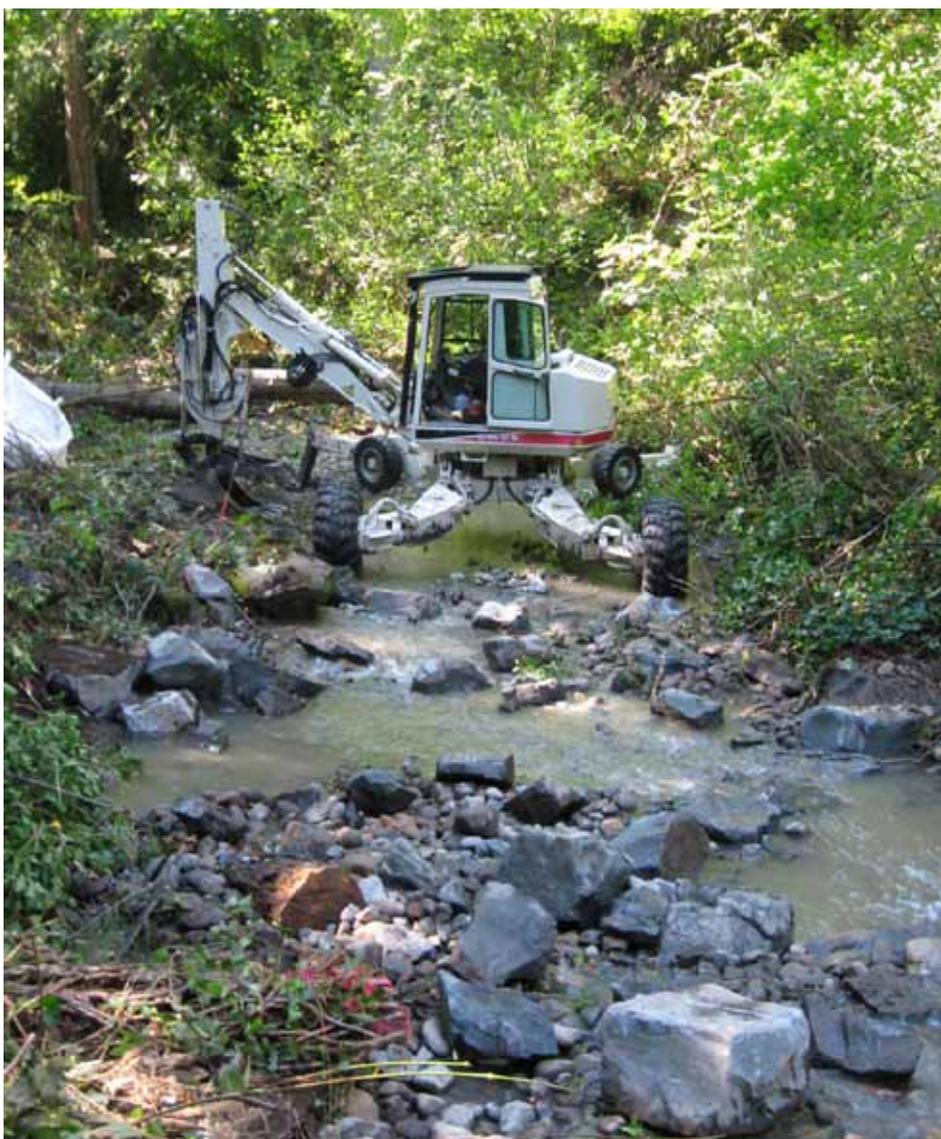
The Spyder Hoe excavator was chosen for its ability to “walk” up the creek channel with minimal environmental disruption. PACE Engineers/SWSSD
